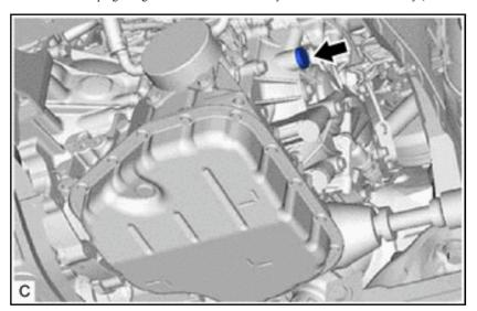
b. Add fluid to the refill hole using the correct amount of fluid as listed in the table below.
