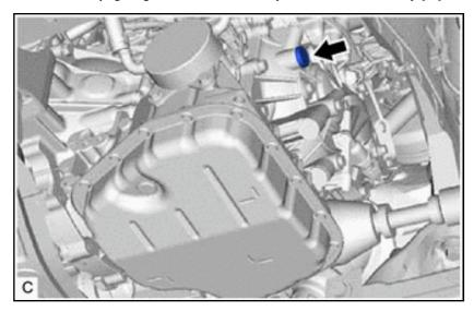
$d.\ Using\ a\ 6\ mm\ hexagon\ socket\ wrench, remove\ the\ overflow\ plug\ and\ gasket\ from\ the\ continuously\ variable\ transaxle\ assembly.\ [*3]$
