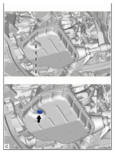
f. Temporarily install the gasket and overflow plug to the continuously variable transaxle assembly.
