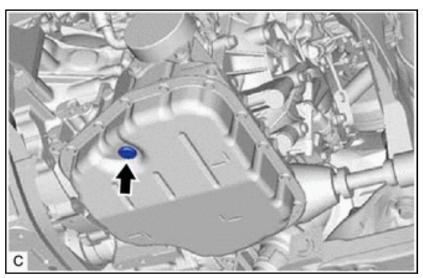
e. Using a 6 mm hexagon socket wrench, remove the No. 1 transmission oil filler tube from the transaxle oil (CVT) pan sub-assembly and drain the fluid. [\*4]
