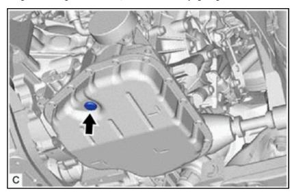
WARNING: Be careful as the fluid coming out of the overflow plug hole is hot.
