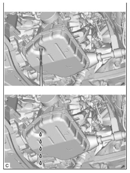
The fluid flow will not stop completely because the fluid continues to expand as its temperature increases.
