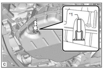
h. Temporarily install the gasket and overflow plug to the continuously variable transaxle assembly. [\*7]
