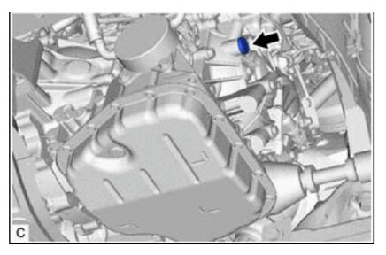
Reuse the old gasket as the refill plug will be removed again to adjust the fluid level.
