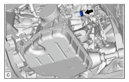
b. Using a 6 mm hexagon socket wrench, remove the overflow plug and gasket from the continuously variable transaxle assembly.
